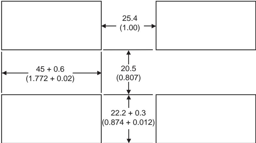
From the front of the panel, slide the housing through the cutout. The housing gasket should be flat against the housing flange before installing.
