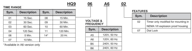
60 cycle units can be used for 50 cycle application; however, the motor will run at 5/6 speed
