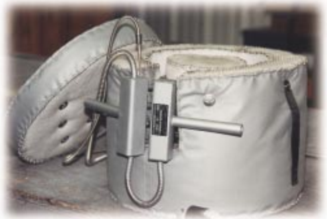
Laboratory test tank with high heat capacity and high temperature capabilities. Note specialized insulation package.
