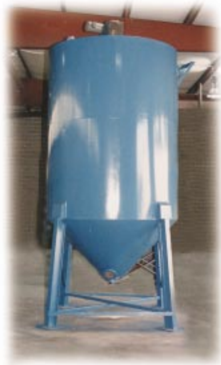
Jacked Heated Hopper has both an inner and outer wall. A heat transfer fluid was circulated through the space between these walls. The flanged connections and the Hot Oil System are not shown.
