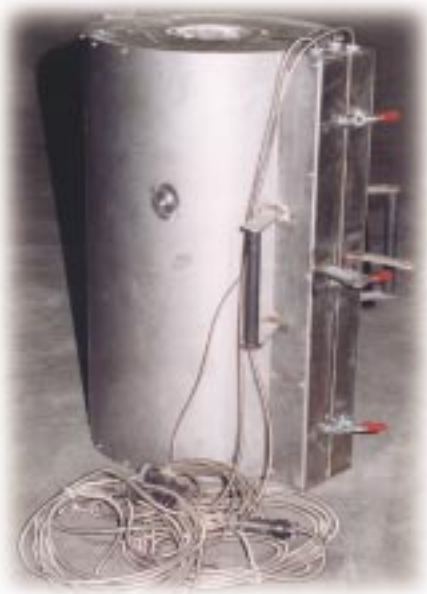
Clam shell heaters used for heating candle filters on an extruder line. 12 kW total.
